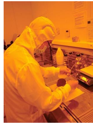
Fig. 3 Fabrication of diaphragm pressure sensors on a Si wafer.
